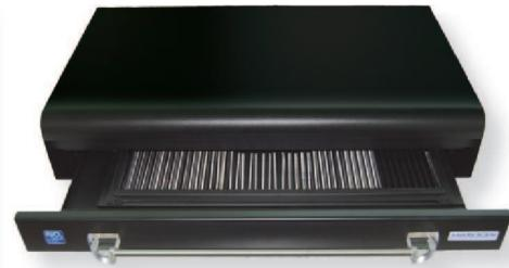
2b. Scanning of test strips in the incubation tray with the BTR48
